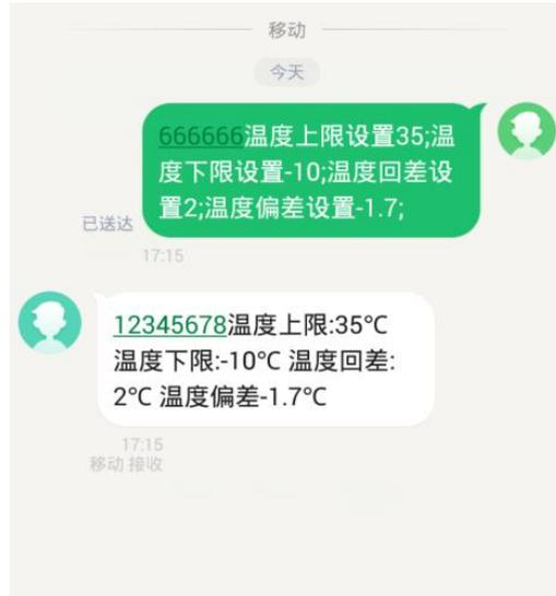
将温度上限关联 1 号继电器，温度下限关联 2 号继电器
